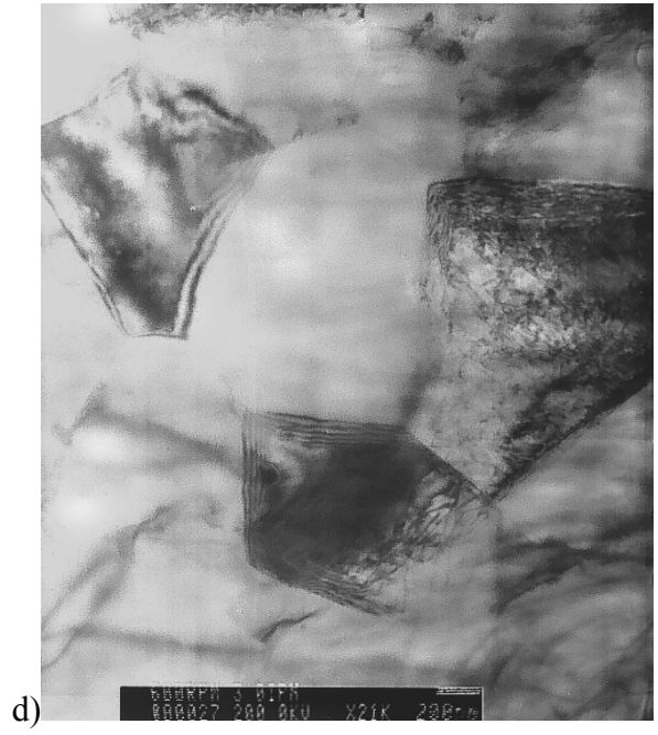
Figure 4-13 a) Optical microscope picture of as received AA 5052 and TEM pictures of FS processed AA 5052 at 600rpm and b) 1.5, c) 2.5 and d) 3.0 in/min
