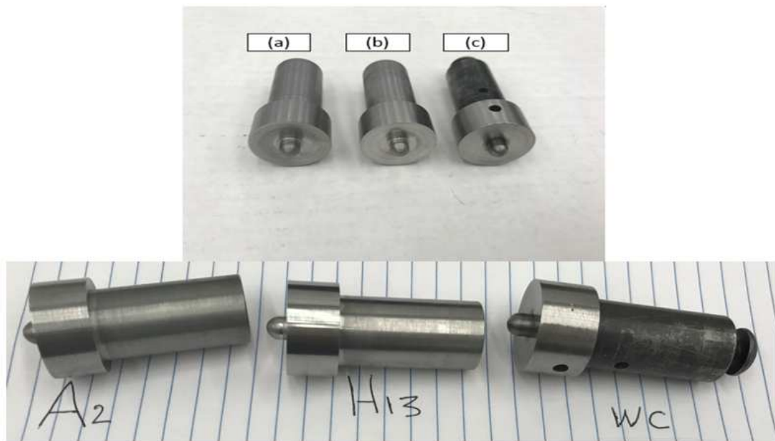
Figure (3.2) (a) and (b) are fixed tool, and (c) the adjustable tool
