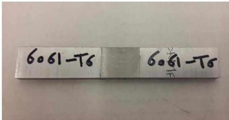
Figure (4.3) Al (6061-T6) specimen
