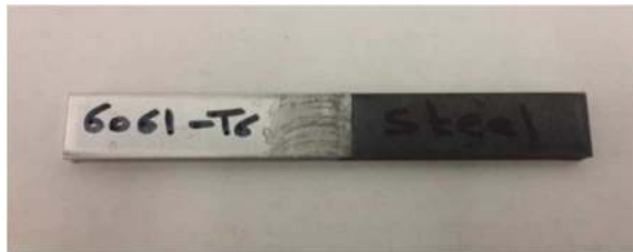
Figure (4.47) Friction stir welding specimen between Al (6061-T6) and (1018 steel)
