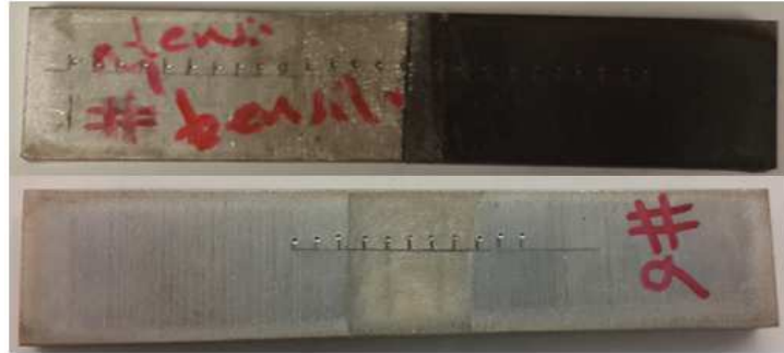
Figure (3.4) Shows the specimen hardness which illustrate the position and the distance between each two points (3mm).
