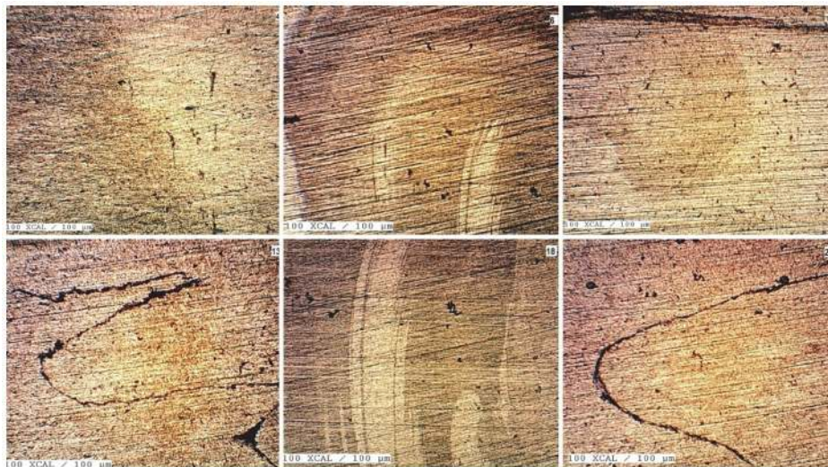
Fig. 5. SEM optical microstructure and texture of cross section of different welding joints
