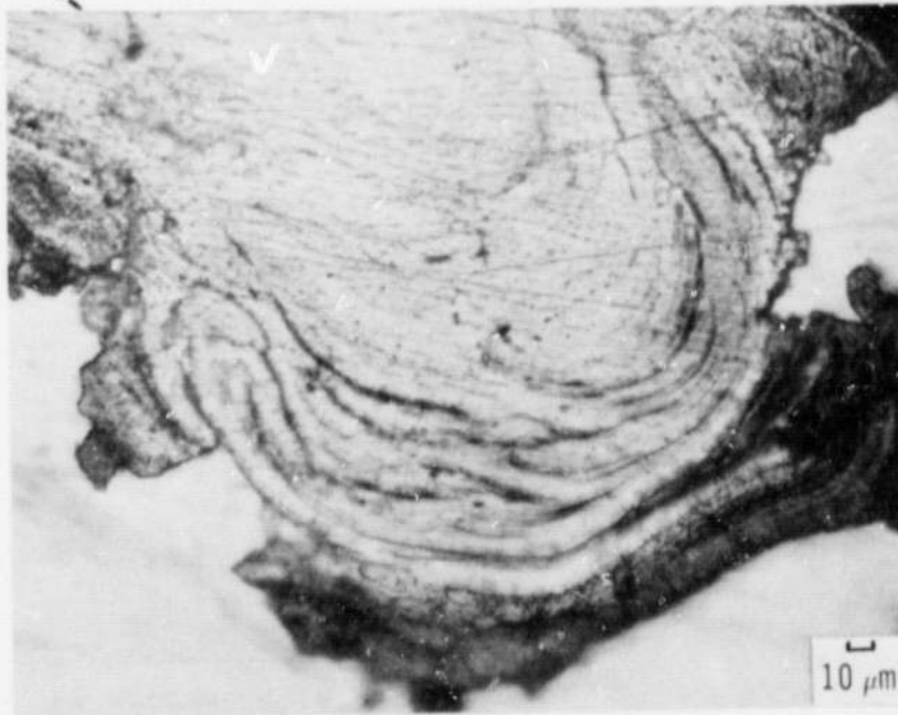
Figure 7. - Rider transfer film after 3.2 kc of sliding for a pin which slid on an UHMWPE disk at 1 rpm.
