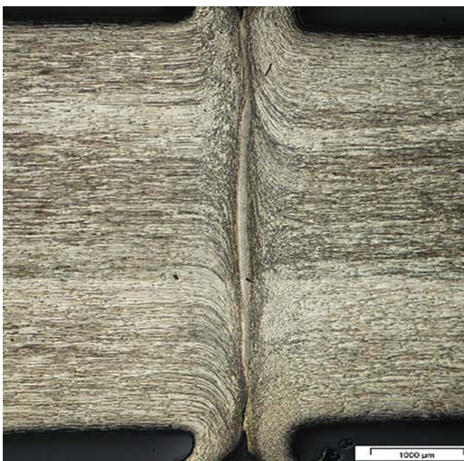
Fig. 7. Microstructure of friction welded joint of 316L UFG steel, etched
