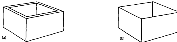
Fig. 4. (a) A box in the trihedral world and (b) a box in the Origami world.
