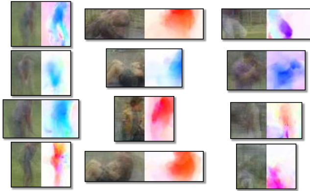
Figure 2. Example part clusters for (left-to-right) golf swing, sit up and baseball pitch, shown as the average of the color image (left) and optical flow (right) for a single frame. The consistent part alignments inside each cluster are exemplified by the sharpness in the color and motion images. This alignment leads to better classifier detection performance.
