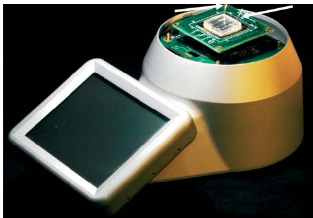
Fig. 8 A photograph of the LOC system in configuration to test the nanowire based sensors with microfluidics channel as per the design in Fig. 6. The fluid was delivered to the system by the tubes connected to the chip through the PDMS cap as shown by the arrows.
