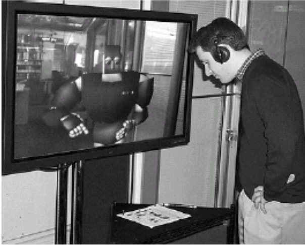
Figure 3: MACK was designed to study face-to-face grounding [19]. Directions are given by the avatar using a common map placed on the table which is highlighted using an over-head projector. The head pose tracker is used to determine if the subject is looking at the common map.
