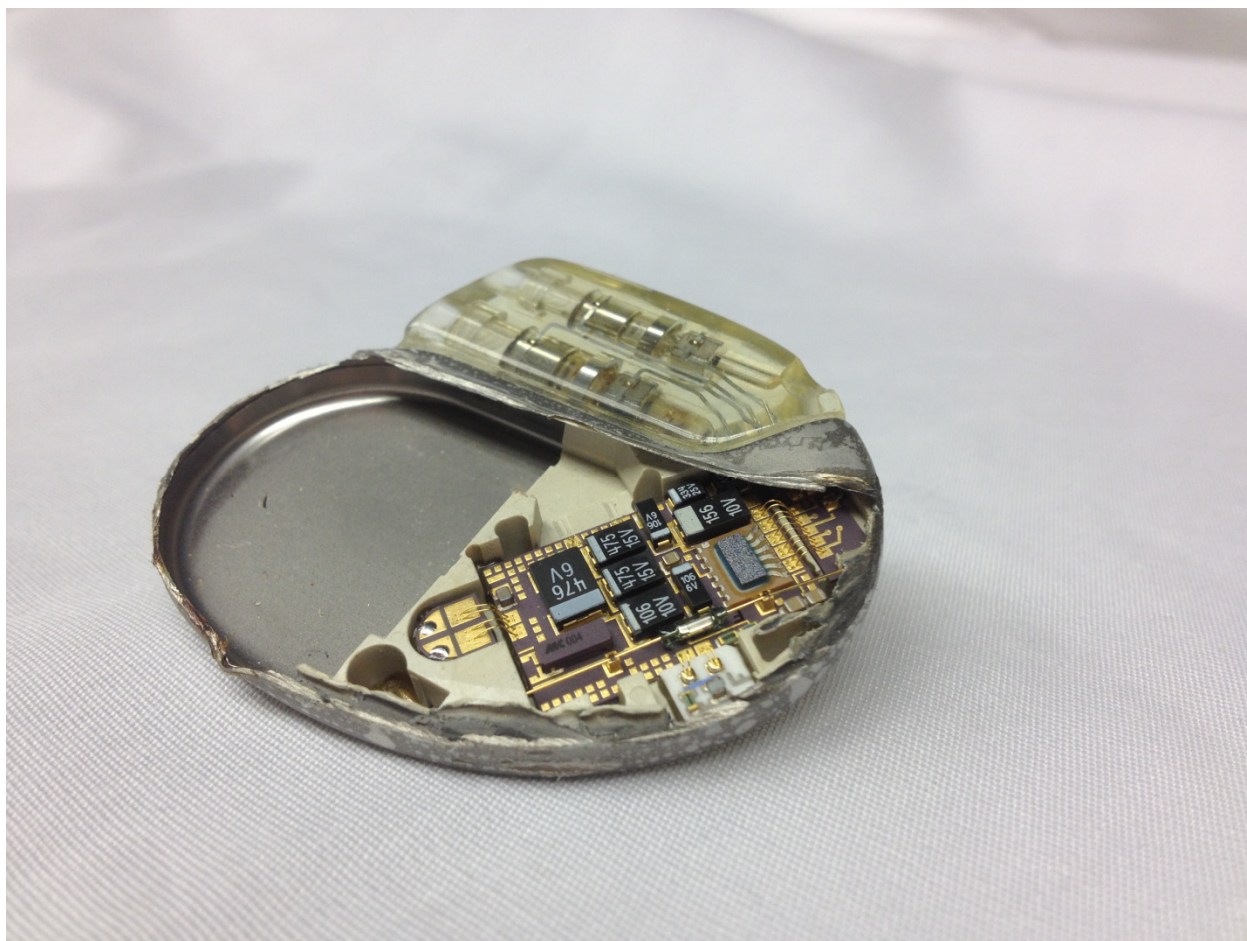
The open pacemaker prior to its wiring to the external power source
