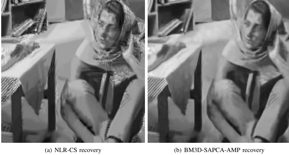
Fig. 17. Reconstructions of 10% sampled 256 \times 256 Barbara test image with additive white Gaussian measurement noise with standard deviation 30. Note that BM3D-SAPCA-AMP exhibits far fewer artifacts than NLR-CS.
