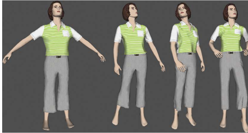
Fig. 10. Animation from one posture to another allows testing the fitness and the comfortability of a garment.
