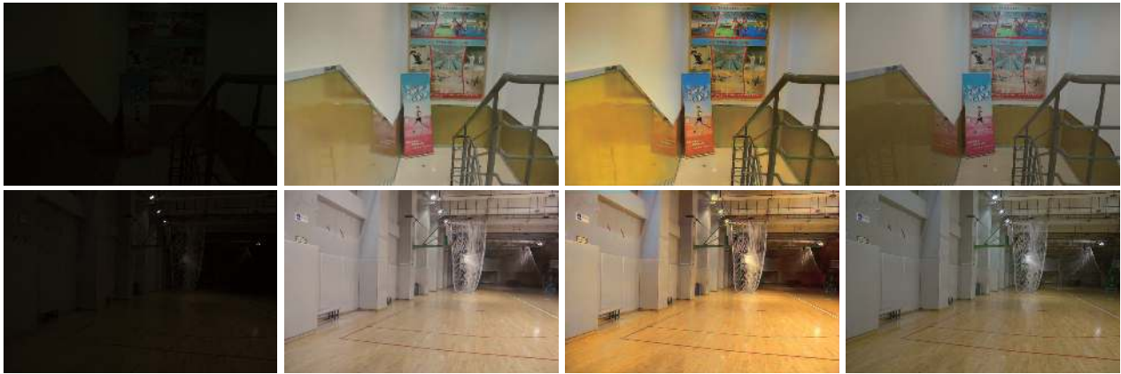
Figure 5. The first to fourth panels: low-light image, the result without perceptual guidance, the result with perceptual guidance, normal light image.
