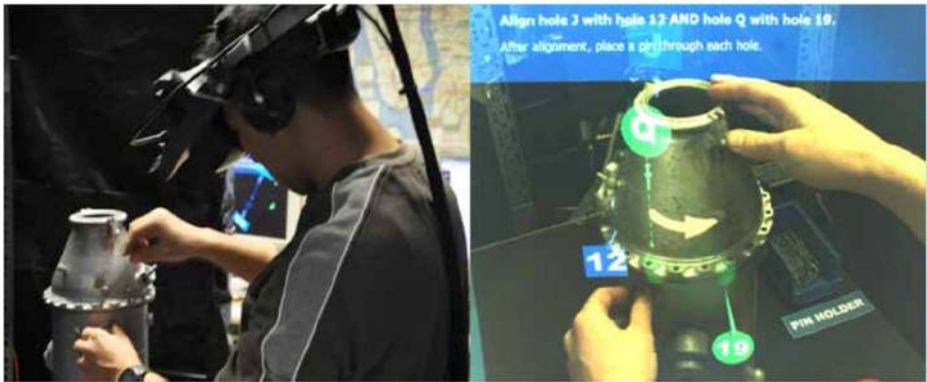
Fig. 5 Experimental Augmented Reality Assistance for an Aircraft Engine Assembly Task. Head tracked optical see-through head-worn display overlays graphics on the user's view of components to be assembled. View through the head worn display shows dynamic 3D avatars and labels that provide assistance in spatially aligning components [48]. (Best in color)
