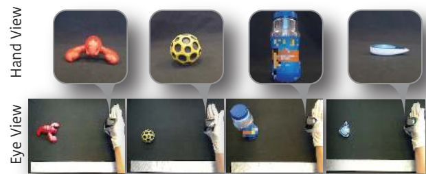
Figure 2: Eye-view images were captured by a webcam (Logitech Webcam C600, 1600×1200 resolution) for labelling and corresponding hand-view images were captured by GoPro (GoPro Hero Session, resolution of 3648×2736 pixels) for training.
