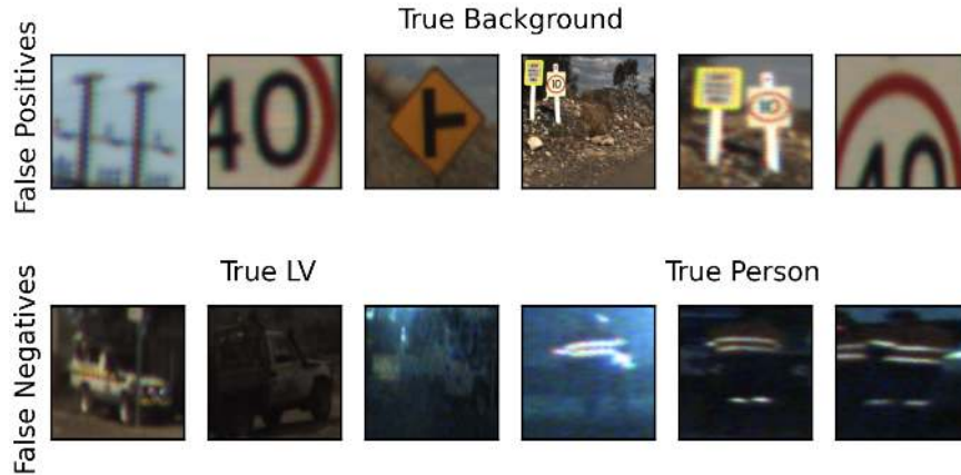
Fig. 7 Validation samples where the background model failed. Images are shown in their warped form, representing the ConvNet input. The four right false negatives were collected at night.
