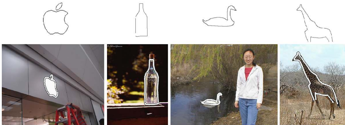
Fig. 18 Detection from hand-drawn models. Top : four of the five models from Ferrari et al. (2006). There is just one example per object class. Bottom : example detections delivered by our shape matching procedure, using these hand-drawings as models
