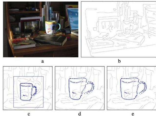
Fig. 8 Object detection. (a) A challenging test image and its edgemap (b) The object covers only about 6% of the image surface, and only about 1 edgel in 17 belongs to its boundaries. (c) Initialization with a local maximum in Hough space. (d) Output shape with unconstrained TPS-RPM. It recovers the object boundaries well, but on the bottom-right corner, where it is attracted by the strong-gradient edgels caused by the shading inside the mug. (e) Output of the shape-constrained TPS-RPM. The bottom-right corner is now properly recovered
