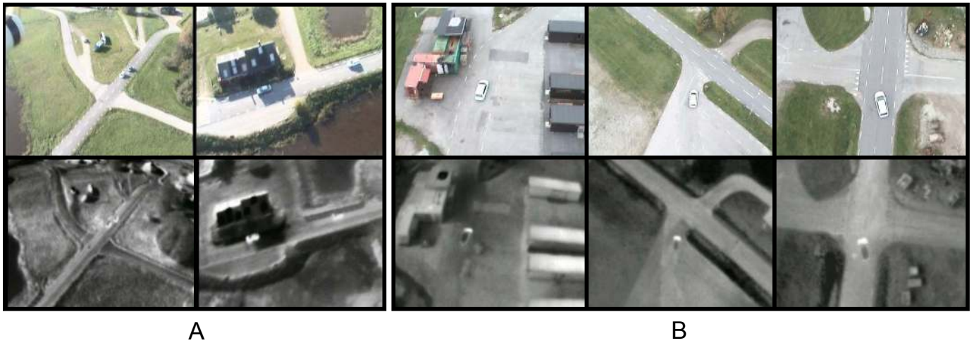
Fig. 3. A. Two frames from video sequence with the UAV hovering close to a road segment observing two cars performing overtaking maneuver. B. Three frames from video sequence with the UAV following a driving car passing road crossings. Top row contains color images and bottom row contains corresponding thermal images.
