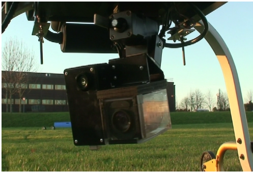
Fig. 2. Onboard camera system consisting of color and thermal cameras mounted on a pan-tilt unit.
