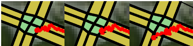
Fig. 4. An example where noise makes it look like a car enters a crossing twice. Each red dot is an observed car position.
