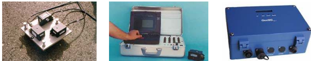
Figure 11. (a) Force balance accelerometers; (b) Multi-channel data acquisition and processing system for ambient vibration tests; (c) Strong motion tri-axial seismograph
