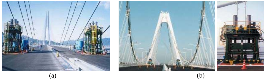
Figure 10. Forced vibration tests of (a) Tatara cable-stayed bridge ( http://www.hsba.go.jp ) and (b) Yeongjong suspension bridge ( http://www.yeongjongbridge.com )
