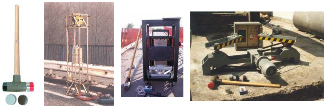
Figure 1. a) Impulse hammer; b) Impulse excitation device for bridges (K.U.Leuven); c) Electrodynamic shaker over three load cells; d) Eccentric mass vibrator.
