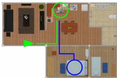
Figure 3: An example task. The green segment corresponds to the solution of a NAV task, "go to the cup", where the cup is circled in green. The green plus blue segments represents a path for the PICK task, "move the cup to the bed", where the bed is circled in blue.
