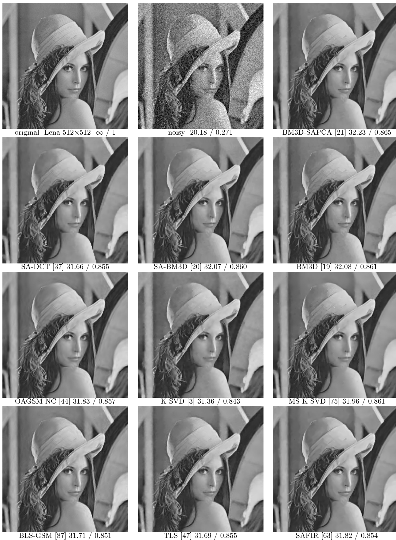
Fig. 10 Denoising of Lena corrupted by noise with \sigma = 25 . The two numbers reported under each image are the corresponding PSNR and MSSIM values.
