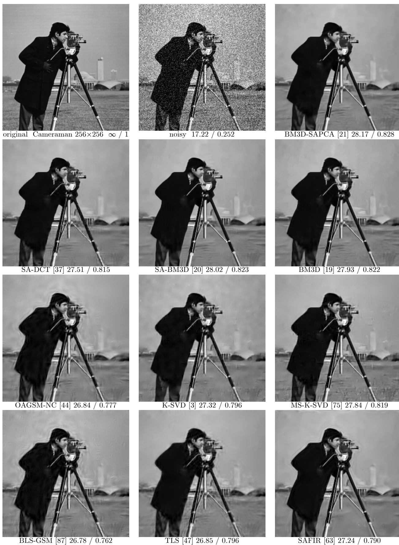
Fig. 11 Denoising of Cameraman corrupted by noise with \sigma = 35 . The two numbers reported under each image are the corresponding PSNR and MSSIM values.
