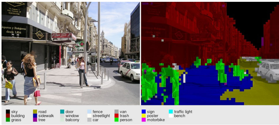
Fig. 11 Sample output of the scene labelling system described by Grangier et al. (2009). This large convolutional network gives good recognition accuracies but very coarse segmentations
