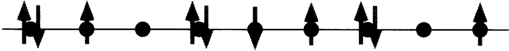
Fig. 2. An allowed configuration in a tight-binding model with a single orbit per site. Each site in the lattice can be either empty, singly occupied by an electron with up or down spin, or doubly occupied by electrons with opposite spins. If we consider the Hubbard type interaction, we get an extra energy U > 0 whenever two electrons occupy a single site. (See §2.5.) The interaction energy for the above configuration is therefore 3U .
