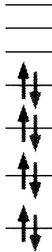
Fig. 3. Schematic picture of the ground state of a non-interacting many-electron system. The lowest N_e/2 single-electron energy levels are “filled” by both up spin and down spin electrons. The state naturally exhibits paramagnetism known as ‘Pauli paramagnetism.’
