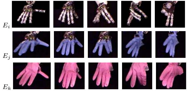
Fig. 9 Examples of multi-view models of three entities characterizing different appearances of the hand of the robot (each model with its views is shown in one line).
