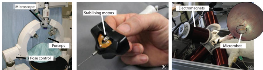
Fig. 3. Retinal surgery requires impressive dexterity and micrometre accuracy. Surgical platforms range from (a) large-scale remote-centre-of-motion teleoperated systems that replicate and scale clinician's motion: image adapted from Mitsubishi et al. , [104], to (b) hand-held stabilizing tools that increase surgical performance by measuring and filtering hand tremor: image adapted from Riviere et al. , [79], and (c) wireless electromagnetically navigated microdevices for drug delivery: image adapted from Nelson et al. , [105].
