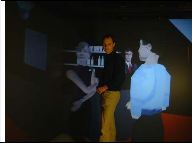
Figure 2b – When the projectors are on the person may be transported into a different world, here interacting with virtual characters in a party scenario.
