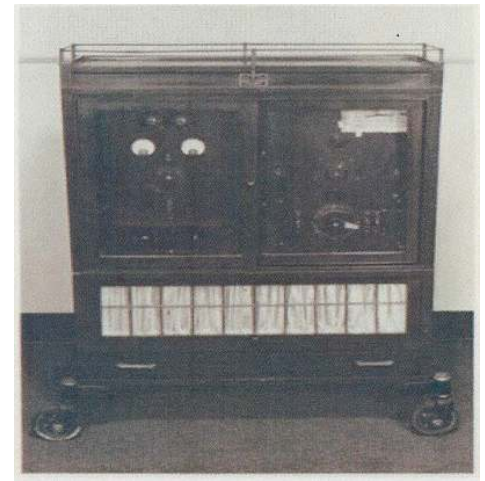
Figure 10. Western Electric IA audiometer, the first widely used audiometer for testing hearing impairment.
