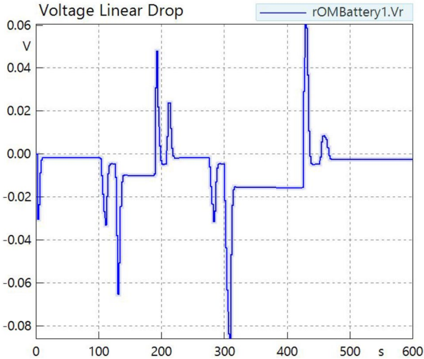
Fig. 27 Voltage drop produced by the internal resistance in a cell during the simulated. itinerary
