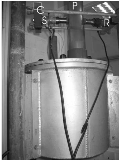
Fig. 4. The author (with students G. T. Yim and M. D. Simpson) invented an ultrasonic device for the detection of bubbles in the opaque liquid “casting slip” which is used by the pottery industry. The detector consists of ultrasonic source (S) and receiver (R) transducers mounted across from each other on the pipe (P). The system is held in place by a clamp (C) which is easily portable, and can be mounted at any position along the pipe, so allowing the operator to track down the source of the bubbles. For further details, including a video of the device in action, see the associated web page. 67
