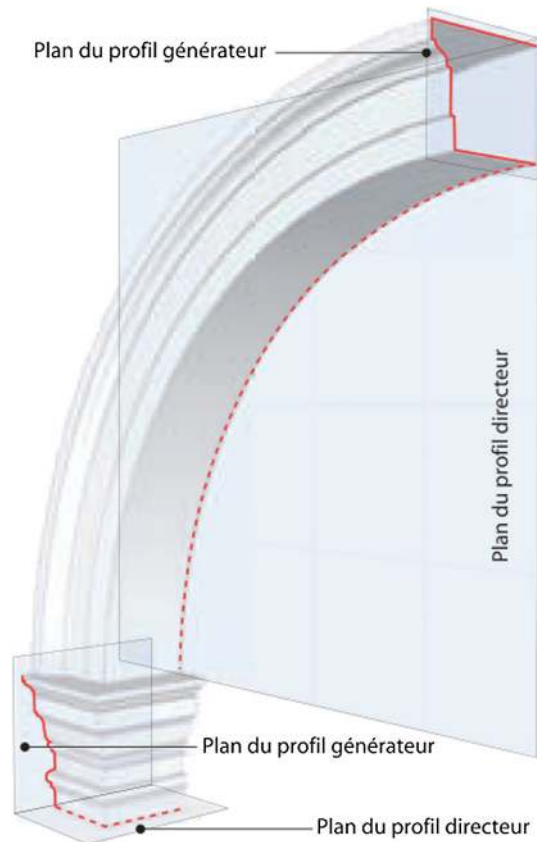
Fig. 6 Evidence of the plan of the generating profile and the plan of the directing path, © Livio De Luca (2006).
