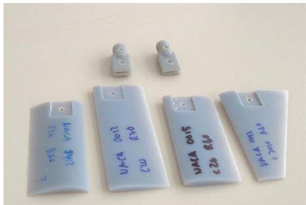
Fig. 4 Different blades with different profiles, length and taper used on the test bench. The blades are manufactured using a rapid prototyping machine
