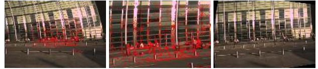
Figure 8: Example of rotation undistortion ( \omega solver). Correspondences are displayed in red. One camera has narrower FOV. Although parts of the wide-angle view have no correspondences, they are undistorted correctly.
