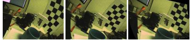
Figure 7: Example of rotation undistortion ( \omega solver) for close-range scenes. The distance to the nearest scene points is \approx 10\times the baseline.
