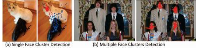
Figure 6: Examples of good face detections from the proposed algorithm. Red fixation points correspond to face and blue corresponds to background. (a) In the presence of salient distracting object (shoe) the face (cat) is reliably detected. (b) We notice that even in challenging scenarios where multiple faces are present, the proposed approach detects reliably. Best viewed in color.
