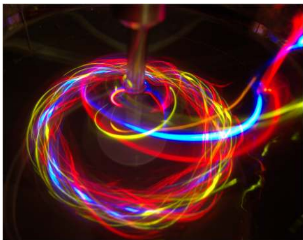
FIG. 55. Long exposure photograph of several finite Stokes number particles moving in the laminar flow of a stirred tank. All particles start in a chaotic flow region but are eventually attracted into a KAM tube where they execute helical trajectories. From Wang, Stewart, and Metcalfe, 2016.
