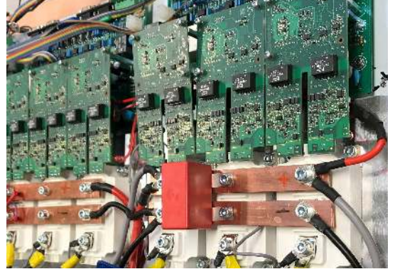
Fig. 9. SiC power module and the driver used in the constructed converter.
