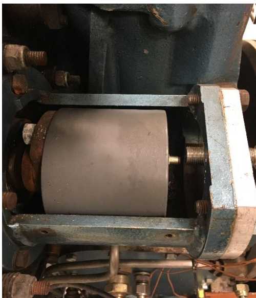
Figure 11: Cam position sensor (Hall Effect Sensor)
