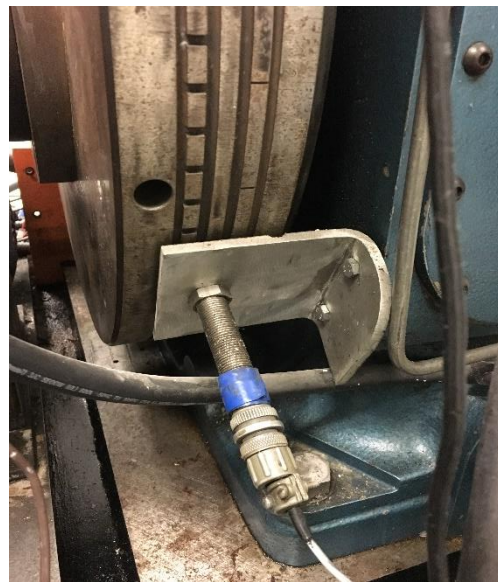
Figure 12: Crank position sensor (VR sensor)
