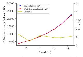
Figure 12. Still water resistance effective power at ballast.
