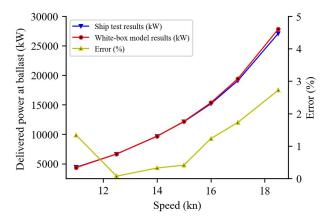
Figure 13. Still water resistance delivered power at ballast.
