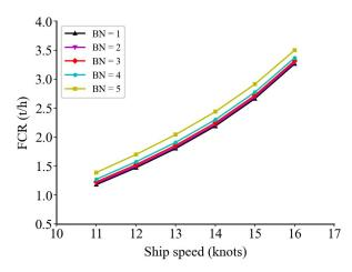
Figure 14. Additional fuel consumption for wind in headwind conditions.
