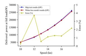
Figure 11. Still water resistance delivered power at full load.
