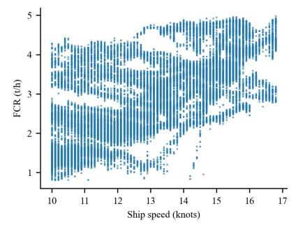
Figure 1. Speed-fuel consumption data distribution after preprocessing.
