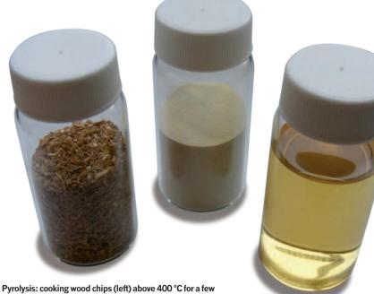
Pyrolysis: cooking wood chips (left) above 400 °C for a few seconds with a catalyst (middle) produces a 'bio-oil' (right).
