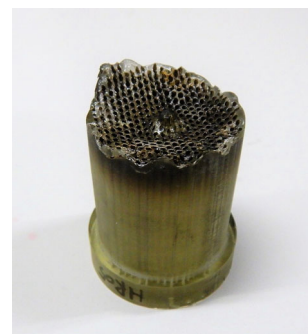
Fig. 28. The side of the fuel after the visualization experiment ( Test 2 )
