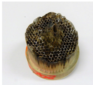
Fig. 31. The side of the fuel after the visualization experiment ( Test 11 )
