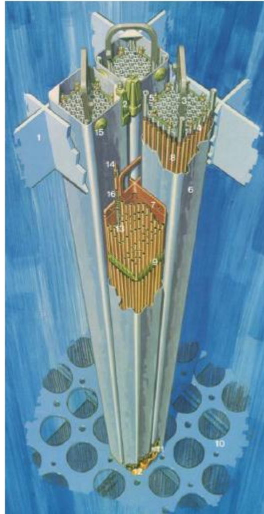
Figure 15. Module of Four BWR Fuel Assemblies and Associated Channel Boxes. (Illustration courtesy of General Electric)
