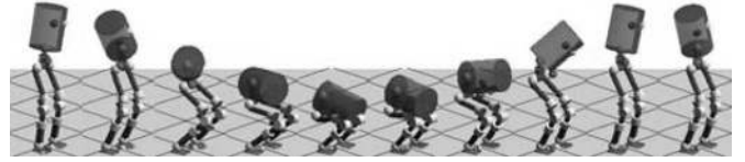
Fig. 5. Animation of a balanced squat with the torso swinging for 1–3 s: the desired CoM height and the torso orientation are simply given by sinusoidal trajectories, but no compensation (42) has been applied.
