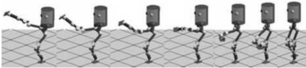
Fig. 7. Animation of a periodic reaching task by a leg with simultaneous balancing.
