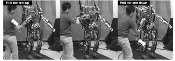
Fig. 11. Experiments on the upper-body interaction with balance. The human shakes the arm. Note that the GAF including the antigravitational force is distributed not only to the legs and the torso, but also to the arms. The robot is responding to the external force by the full-body compensatory motion.
