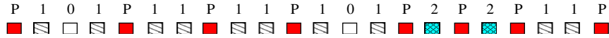
Fig. 3. A valid track assignment solution with a minimum number of power nets ( p_t = 3 ).
