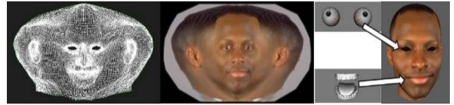
FIGURE 7. The illustration of the UV texture mapping. The first figure is the plane projection of our mesh model, the second figure is the panoramic UV texture generated by our network, the last figure shows the process of the face organic components padding.
