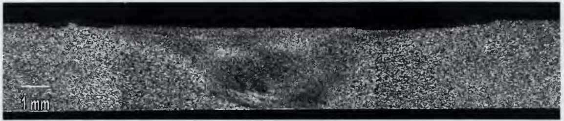
Figure 22: Etched Side Area of a Friction Stir Weld in 5454-O Aluminum. The Weld Nugget can be Seen in the Center with the Heat-Affected Zones on Either Side.
