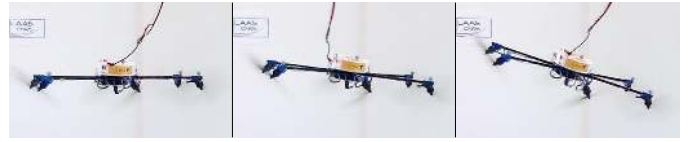
Fig. 4. The Tilt-Hex performing Exp. 1.1 at different time instances: Left t = 15.4 s; middle t = 37.7 s; right t = 47.9 s. Although the reference orientation is constant and horizontal the Tilt-Hex adapts its orientation to allow for following the reference position.
