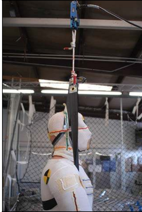
Figure 10: Seatbelt straps with brass grommets on the ends tied with climbing rope and attached to solenoid dropping mechanism.
