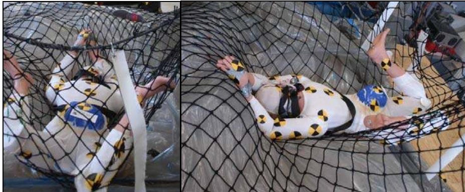
Figure 20: Preliminary tests showing final position of dummy in the catching mechanism: along track view (left) and side view (right).
