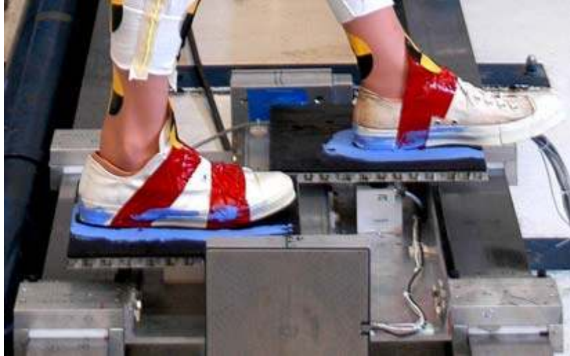
Figure 14: Pedestrian sled platform.
