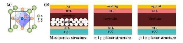
**Figure 1.** (a) The crystal structure of the ABX<sub>3</sub> perovskite material. Reproduced with permission.<sup>[7]</sup> Copyright 2014, American Chemical Society. (b) Device structures of perovskite solar cells.
