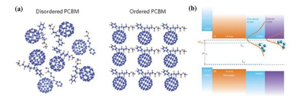
**Figure 4.** (a) Schematic of disordered and ordered  $PC_{61}BM$  structures. (b) Schematic illustration of how energy disorder of the  $PC_{61}BM$  layer influences the device  $V_{oc}$ . Reproduced with permission. [65] Copyright 2016, Nature Publishing Group.
