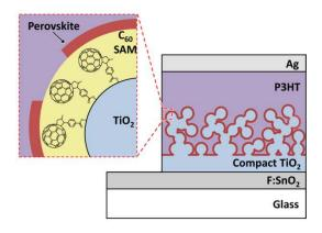
Figure 6. Schematic of device structure and the binding of  $C_{60}$ -SAM to  $TiO_2$  surface.
