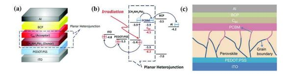
**Figure 2.** (a) The device structure of p-i-n perovskite solar cells. (b) Scheme of the energy levels of each layer in the device. Reproduced with permission.<sup>[54]</sup> Copyright 2013, Wiley-VCH. (c) Schematic device structure of PSCs showing the diffusion of fullerene into the perovskite grain boundaries. Reproduced with permission.<sup>[62]</sup> Copyright 2014, Nature Publishing Group.
