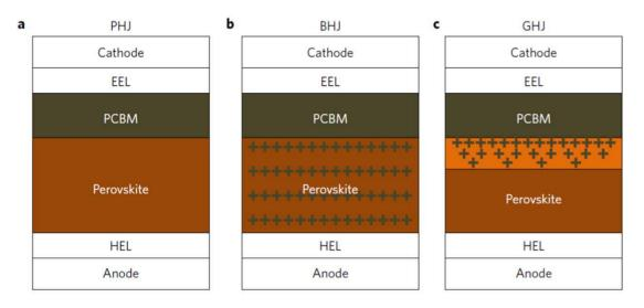
**Figure 9.** Schematic of three types p-i-n PSCs. (a) Planar heterojunction, PHJ. (b) Bulk heterojunction, BHJ. (c) Graded heterojunction, GHJ. Reproduced with permission. [140] Copyright 2016, Nature Publishing Group.
