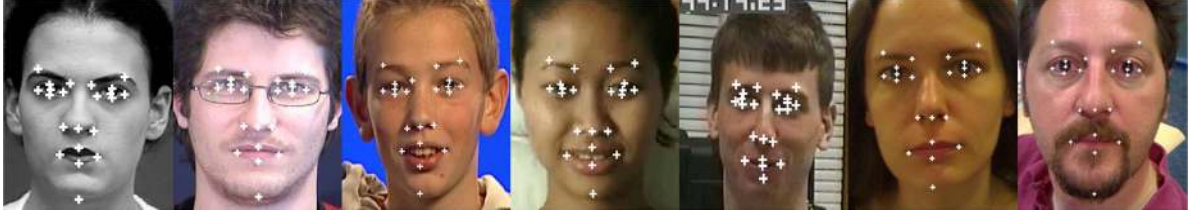
Fig. 4. Typical first-effort results of the proposed facial-point detector for samples from (left to right): CK-db, the MMI database (posed expressions), two images of the MMI database (spontaneous expressions), the triad data set, and two images from a cell phone camera.
