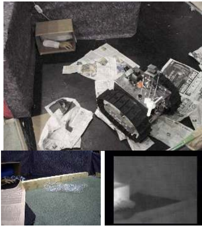
Fig. 3. An autonomously detected victim. The top image shows an overview photo taken by a spectator of the robot after it detected a victim - the arm in the box. The bottom images are the robot's view of a different detected victim. The left image is from the webcam on the robot, and the right image is from the thermocam on the robot.
