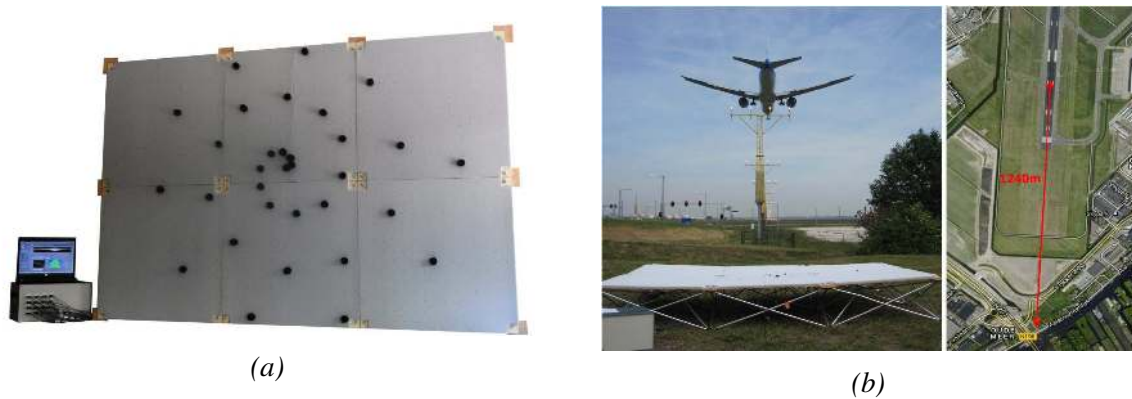
Figure 1: (a) 32 Microphone array configuration in spiral distribution. (b) Experimental set-up located 1,240 m to the South of the threshold of the Aalsmeerbaan (36R) Schiphol airport runway.
